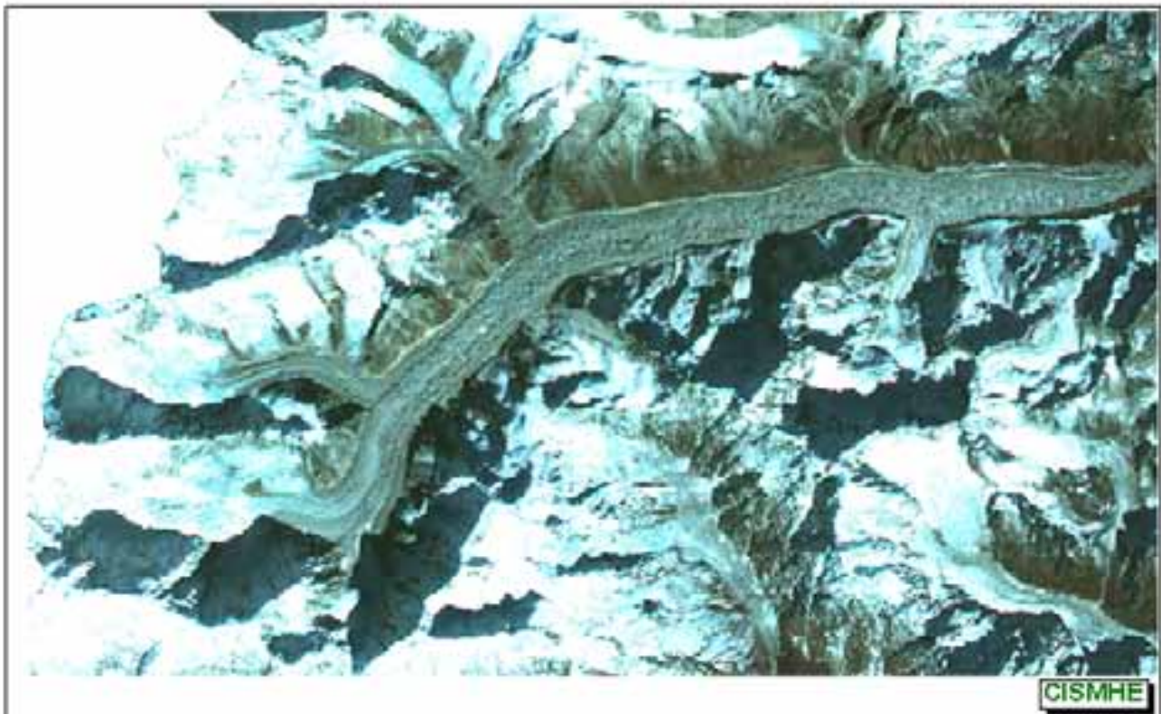
Fig. 3.4 Subset and colour composite bands 9(R), 3(G) and 2(B) of Landsat-7 ETM+ of 26 Dec 2000 to show the ice cover in the Zemu glacier
